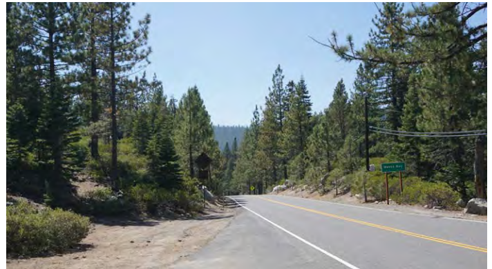
The highway makes an almost 90 degree bend as it enters Meeks Bay which reduces the sight distance for pedestrians crossing the road.
