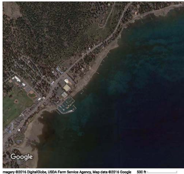
Figure 1: Using aerial imagery along with field verification from a boat, each color spectrum of the Lake is matched to a corresponding habitat type (boulder, gravel, etc.) to estimate distribution of fish habitat around the Lake. This method allows TRPA to track changes over time using satellite imagery.
