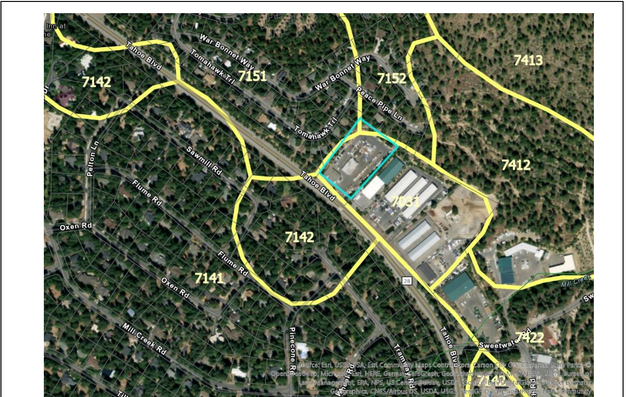
Image 3 – 2007 Soil Survey mapunits in yellow. The parcel remains mapped as 7031- pits and dumps mapunit. The area where UmE, Umpa 15 to 30 percent slopes (Class 3) was mapped is now mapped as 7151- Jorge 5 to 15 percent slopes (Class 6) and 7152- Jorge 15 to 30 percent slopes (Class 4). Mapunits 7142 – Inville 9 to 15 percent slopes (Class 6) and 7141-Inville 2 to 9 percent slopes (Class 6) are mapped below the parcel. Mapunit 7422- Cassenai- 15 to 30 percent slopes (Class 4) is mapped to the southeast of the pits mapunit.
