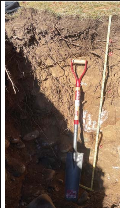
Photo A – View of soil profile showing bottom depth of 60 inches. Fine root penetration to bottom. No indication of seasonal water table.
