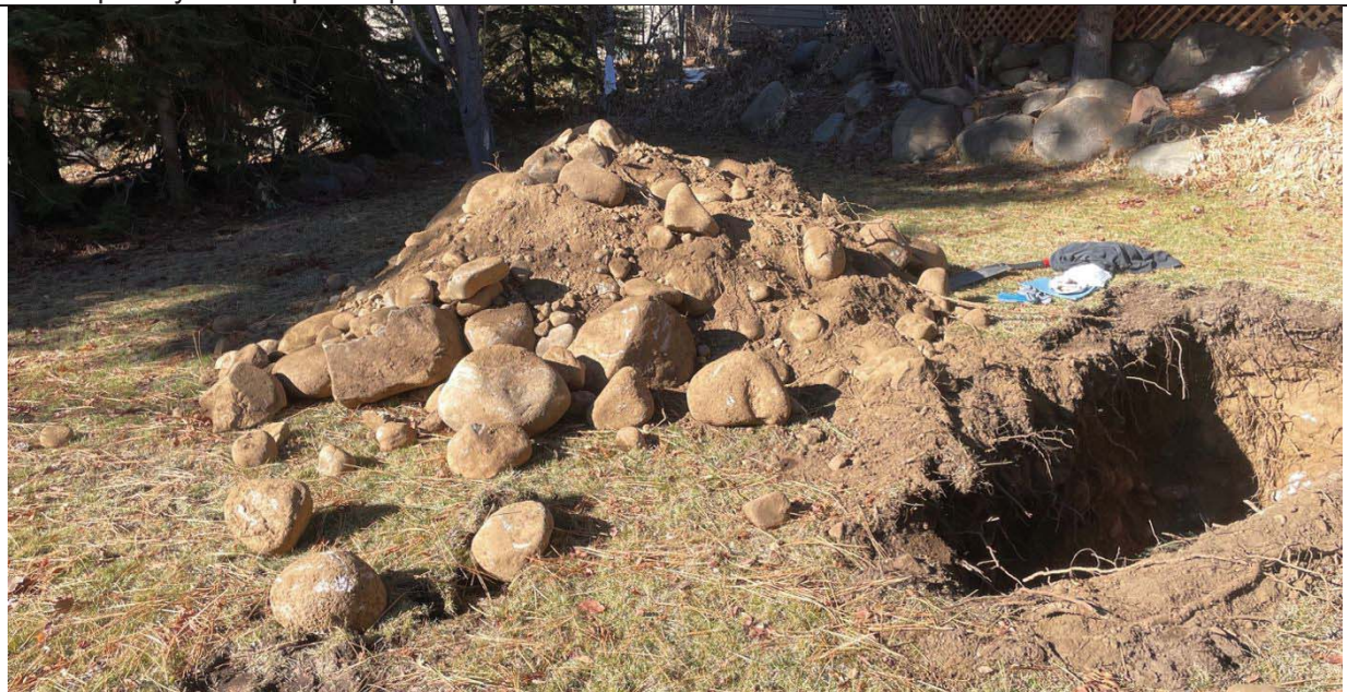
Photo 4 – View to northwest at south portion of parcel where Test Pit no. 1 was excavated by backhoe. The pit was located about 35 feet north of Edgewater Drive and 40 feet east of the west property line. Slopes are 9% in this vicinity. Side cast material for the test pit shows the rounded stones and boulders that increase with depth (no root restriction nor evidence of seasonal water table).
