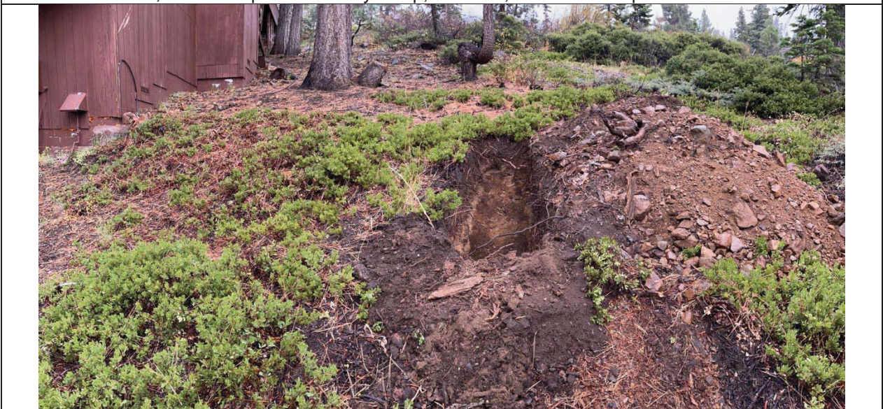
Photo 6 – View to northeast toward Test Pit no. 2, located about 20 feet northeast of the residence. The slope in this vicinity is 29%, which was measured on the adjacent (vacant) parcel at right edge of photo. The land surface immediately surrounding the residence is irregular, presumably a remnant condition after house construction.
